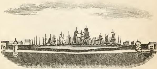
LONGITUDINAL SECTION OF THE THAMES TUNNEL, Showing its course under the River.
